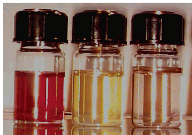
Figure 5. Uptake of \text{HAuCl}_4 into QS-12-S, dispersed in toluene, by liquid-liquid phase transfer (top); starting concentration of \text{HAuCl}_4 in the water phase: c = 10.7 mmol/L (left), c = 53.7 mmol/L (right). Bottom: pictures of toluene dispersions of QS-8-S after filling with metal salt by liquid-liquid phase transfer and subsequent reduction. From left to right: gold, silver, palladium.
